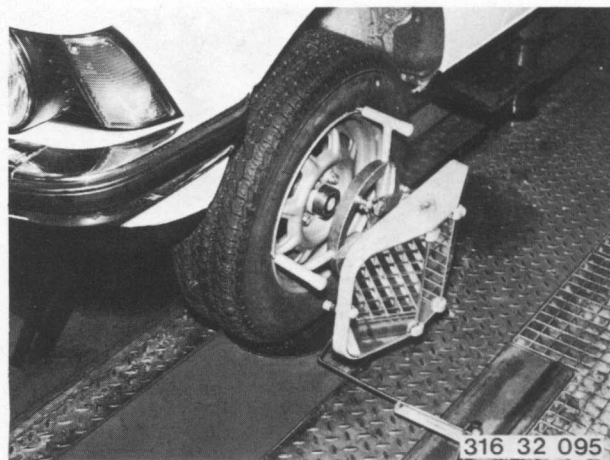
20° left-hand lock measured on right wheel
