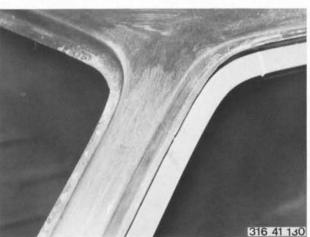
Align and grind both rain moldings. Tin and grind mating surfaces at front corners of outer roof panel. Tin and grind mating surfaces at rear corners of outer roof panel.  $% \left\{ 1\right\} =\left\{ 1\right\}$
