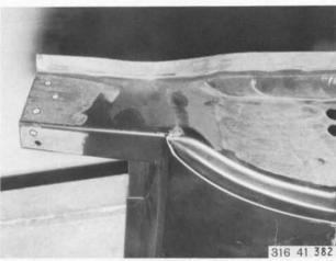
Drill holes for plug welding with shielded arc welder.
