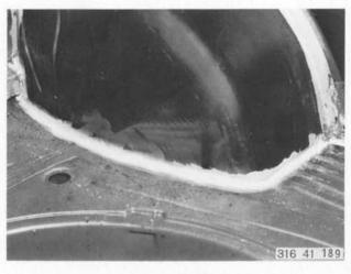
Coat wheelhouse/trunk floor joint with joint sealing compound.
