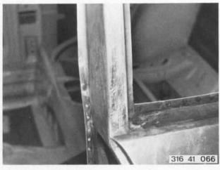
Grind all welding seams. Tin and grind B pillar.
