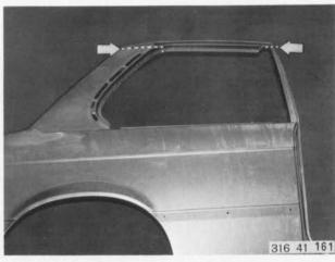
Drill holes in new side panel in area of B pillar for plug welding.
