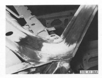
Tin and grind down apron section joints.
