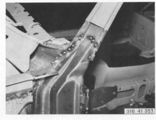
Weld door pillar to side member cover with shielded arc welder.
