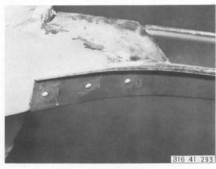
Weld engine carrier to fire wall with shielded arc welder.
