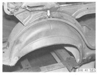
Cut through tank vent pipe welding seam and bend up pipe.
