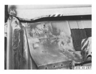
Align mating surfaces and grind bright on both sides. Drill holes for plug welding.
