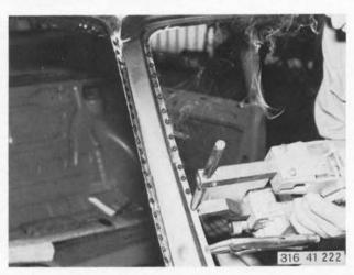
Spot weld apron to window opening and rain molding.
