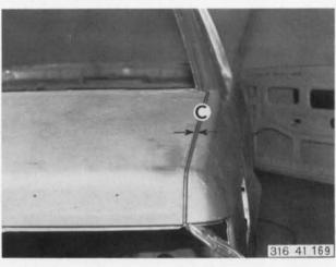
Weld side panel in area of C pillar (shielded arc welding for reinforcement).
