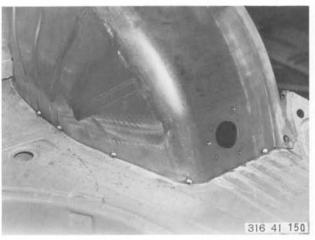
Tack weld wheelhouse inner section.
