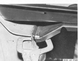
Tack weld wheelhouse to fire wall.
