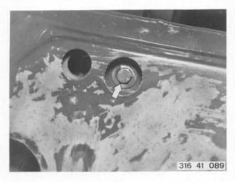
Unscrew upper mounting screw on window guide rails. Remove window guide with window guide rail.
