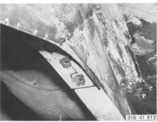
Grind off engine carrier plug welding from below and remove engine carrier.
