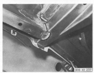
Grind mating surfaces of new left separating wall bright on both sides and coat with zinc powder paint.
