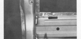
Weld connector plate to longitudinal strut with shielded arc welder.
