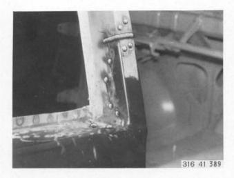
Weld B pillar with shielded arc welder.
