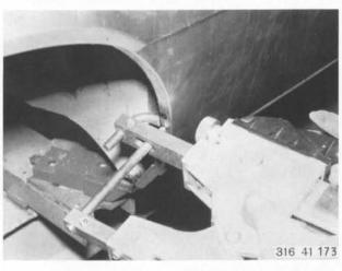
Spot weld side panel to wheelhouse.
