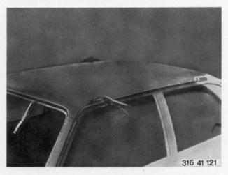
Hold outer roof panel in position with body pliers. Perhaps tack weld in window opening at one point.
