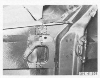
Fit and teck weld connector plate; plug weld in area of reinforcement with shielded arc welder.
