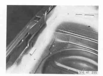
Coat trunk floor/tail panel joint with joint sealing compound and spray with Body Plast.
