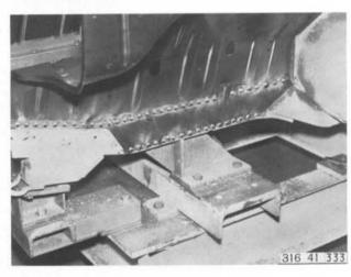
Plug weld wheelhouse to fire wall on inside with shielded arc welder.
