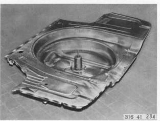
Grind mating surfaces of new trunk floor bright on both sides and coat with zinc powder paint.
