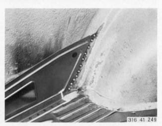
Weld left and right separating walls to wheelhouse with shielded arc welder.
