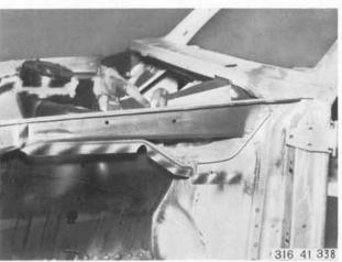
Grind mating surfaces on wheelhouse for connector plate bright.  $% \label{eq:connector} % \label{eq:connector}$
