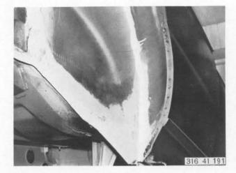
Coat side panel/trunk floor joint with joint sealing compound.
