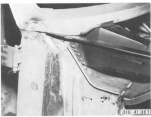
Spot weld wheelhouse to apron and heater separating wall.
