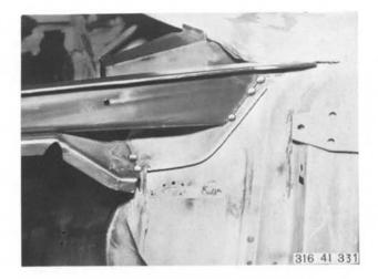
Drill holes in wheelhouse (engine carrier area) for plug welding.
