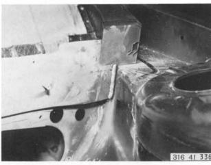
Weld heater separating wall to wheelhouse with shielded arc welder.
