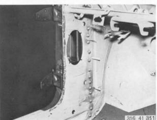
Plug weld door pillar to front edge from inside with shielded arc welder.
