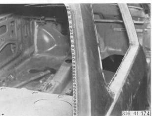
Spot weld side panel to rear window opening.
