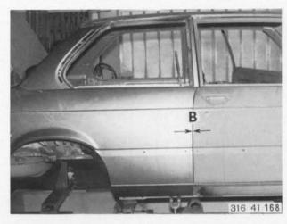
Check gap (C) between side panel and trunk lid, correct side panel location if necessary.
