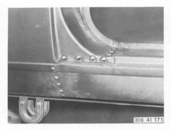
Plug weld side panel in area of entrance with shielded arc welder.
