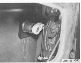
Lift out operating rod between door lock and lock cylinder.
