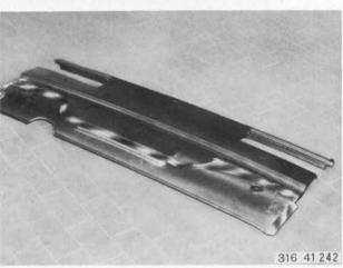
Grind mating surfaces of new tail panel bright on both sides and coat with zinc powder paint.
