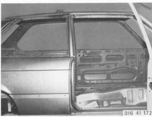
Spot weld side panel in area of side window and door opening.
