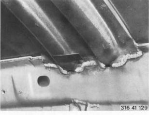
Press roof hoopstick against outer roof panel lightly and weld with shielded arc welder.
