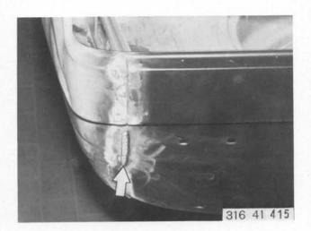
Spot weld side panel in wheel opening.
