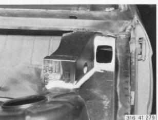
Coat mating surfaces with a joint sealing compound.
