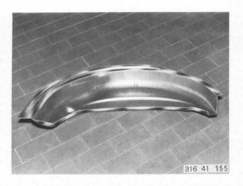
Grind mating surfaces of new wheelhouse outer section bright on both sides and coat with zinc powder paint.
