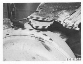
Align and grind bottom mating surfaces bright.
