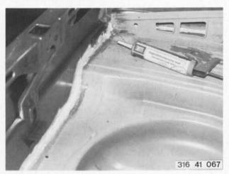
Coat tail panel/side panel joint at trunk floor with joint sealing compound.
