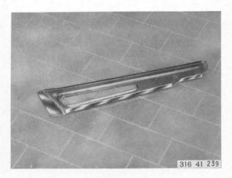
Grind mating surfaces of new right separating wall bright on both sides and coat with zinc powder paint.
