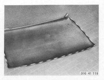
Grind mating surfaces of new outer roof panel bright on both sides.
