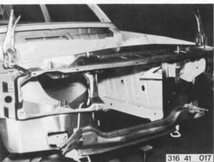
Fit front trim and hold in position with body pliers.
