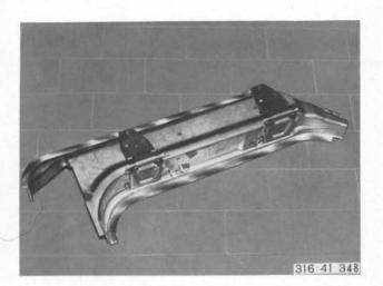
Grind mating surfaces of new door pillar bright.
