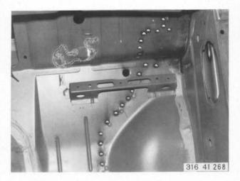
Shield arc weld wheelhouse to fire wall from inside through and through.
