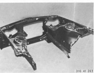
Grind mating surfaces of new front end bright on both sides.
