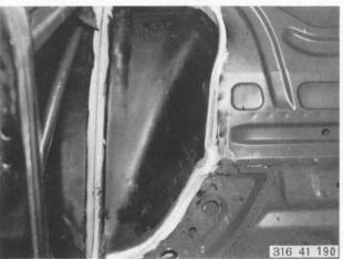
Coat wheelhouse/trunk separating wall joint with joint sealing compound.  $% \label{eq:coat_separating} % \label{eq:coat_separating}$
