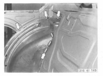
Tack weld wheelhouse inner section.
