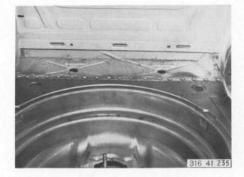
Weld cross member to right side member with shielded arc welder.
