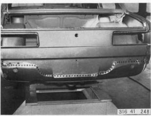
Spot weld tail panel to trunk floor and separating walls.
