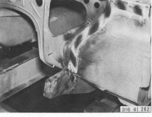
Align mating surfaces and grind bright on both sides. Coat with zinc powder paint.
