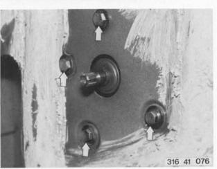
Unscrew window control mechanism mounting screws.
