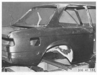
Grind all welded, spot-welded and brazed seams, clean and coat with zinc powder paint.
