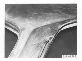
Tin side panel/roof panel joint and grind smooth.
