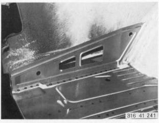
Spot weld left separating wall to trunk floor.
