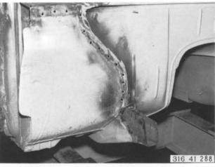
Drill holes for plug welding.
