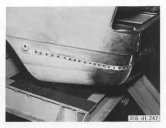
Spot weld trunk floor to left side panel.
