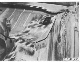
Align mating surfaces and grind bright on both sides.
